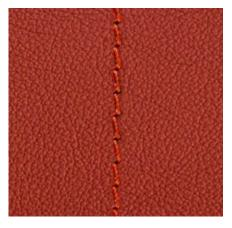
Leather Premium is a relatively smooth cowhide leather with a flat grain and fine top sheen. It is dyed-through and lightly pigmented. The semi-aniline leather is soft to the touch and available in 22 colours.
